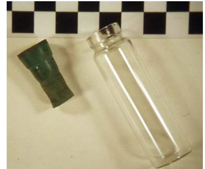
Compressible stopper failure
