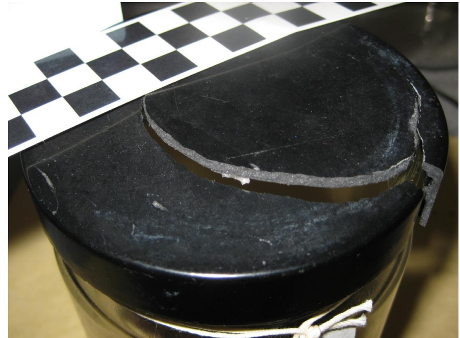
Cracked Bakelite closure
